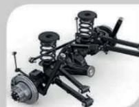
**REAR SUSPENSION WITH COIL SPRING**
